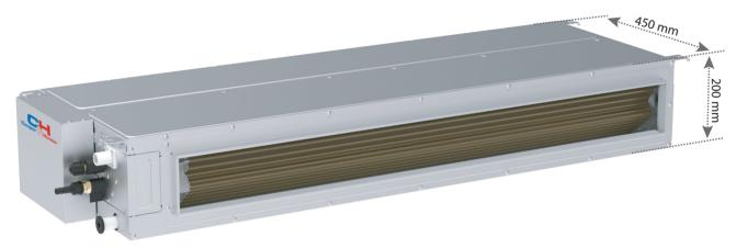
High static pressure duct units ranging from 7 .1 kW to 8.5kW are only 900mm in length. They are suitable to be installed in corridors whose width is  $\leq$  1.2m.
